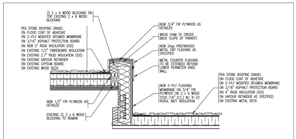
NOTE: EXISTING WOOD BLOCKING TO BE REMOVED ALONG W/ PLYWOOD TO ALLOW FOR INSTALLATION OF NEW KNEE WALL AS DETAILED
