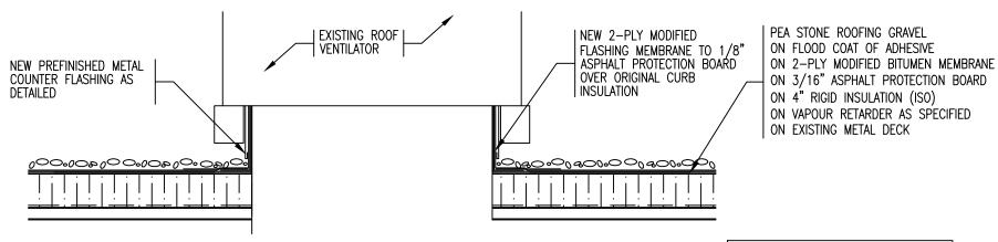
NOTE: ROOF VENTILATOR TO BE LIFTED TO ALLOW FOR BASE FLASHING MEMBRANE ALONG W/ METAL COUNTER FLASHING TO BE INSTALLED ON TOP OF ROOF VENTILATOR
